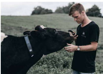
Halter founder and CEO Craig Piggott with a prototype product. The GPS-enabled, solar-powered collar allows a farmer to control a herd remotely via a smartphone, using audio signals.
